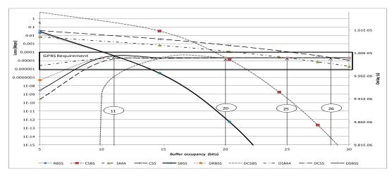
Figure 4: Graph of Loss against Buffer Occupancy
