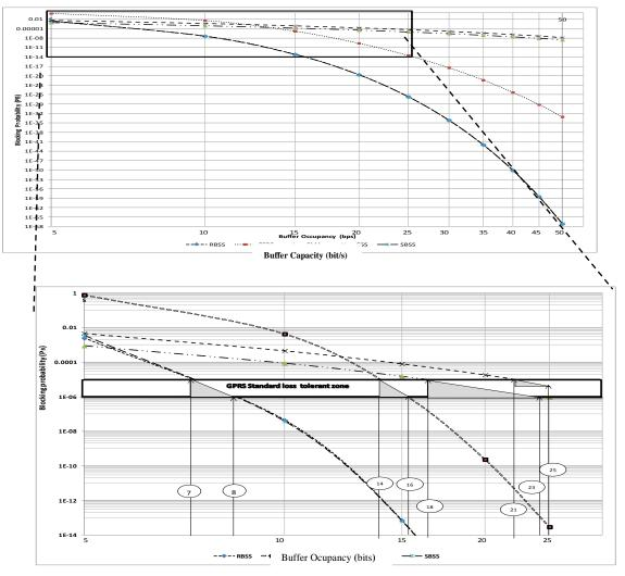
Figure 2: Blocking Probability (P<sub>B</sub>) Against Buffer Occupancy
